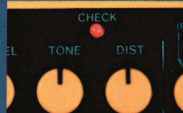
▲LED with battery check function. In early models, the LED lit up only as the effect was turned on, but later models were changed so the LED was always lit when the effect was on.
