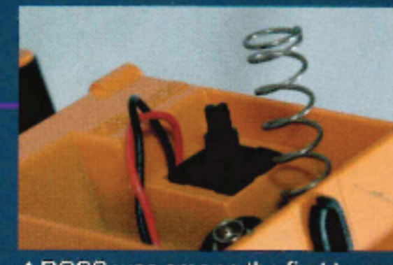
▲BOSS was among the first to use electronic switches. These switches completely eliminate the clicking noise produced by conventional mechanical switches.
