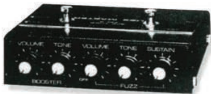
▲The Ace Tone FM-3 Fuzz Master had both booster and fuzz effects built-in.
