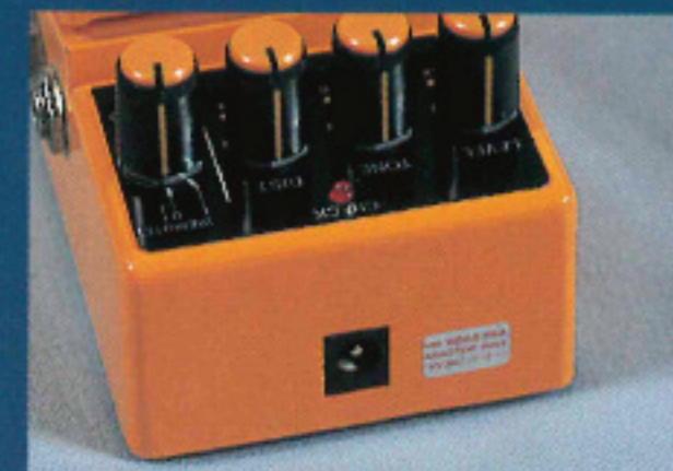
◀BOSS effects are equipped with an AC adaptor terminal to eliminate power supply worries during long performances. This was a revolutionary idea 24 years ago.
